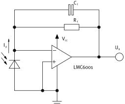
$U_a = I_p x R_f = o \dots \sim V_{cc}$
